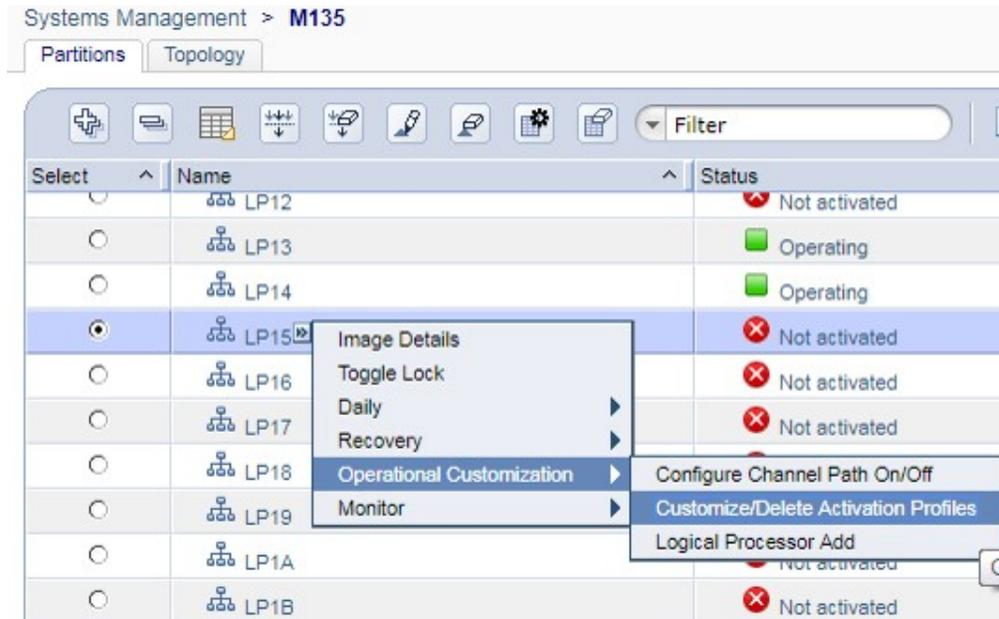
Figure 7. The Partitions window of the HMC
