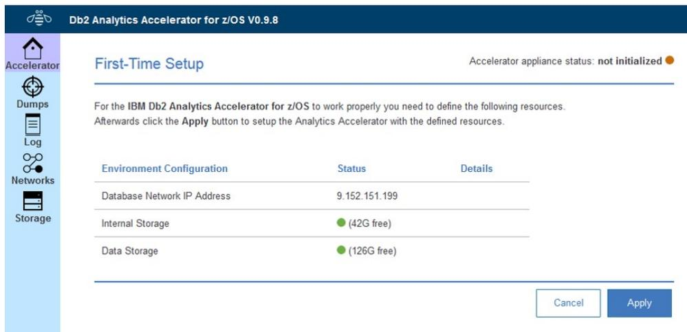
Figure 16. The First-Time Setup window after network and storage configuration
